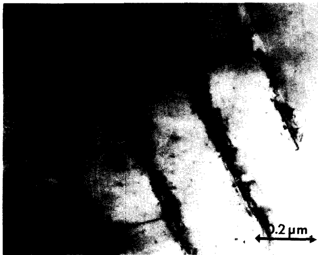
Fig. 3. Thin foil transmission electron micrograph of lamellar structure in cast Pb–0.1wt.%Ca–0.3wt.%Sn alloy, ice-water-quenched and aged for 400 days.
